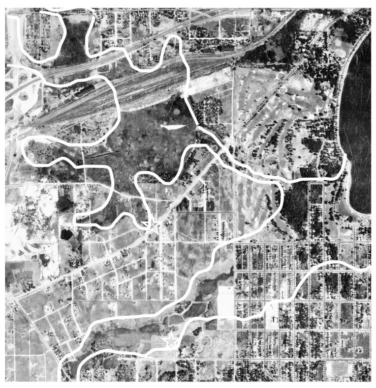
The approximate contour of the swamps taken from a 1901 USGS survey is traced over this aerial photo from 1940. The locations of the new Bridgewater bank headquarters and the new house on Grimes, both requiring deep pilings for foundations are starred. Bass Lake has been filled for the Milwaukee Road rail yards. The edge of Lake Calhoun/Bde Maka Ska is at upper right.
