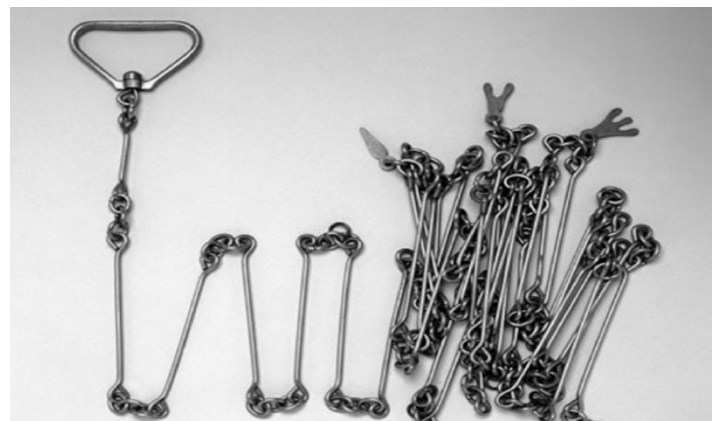
Above, a surveyor's chain, sixty-six feet long. Below, in areas that T.B. Walker did not disrupt with his diagonal Lake Street layout, the original grid records 40-acre plots in 8-block squares.
